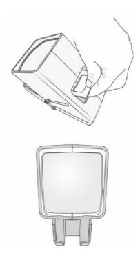
• To release the slide, firmly press and hold the release button. The release button is just above the power button on the right side of the slide viewer. Hold the release button down all the way until the slide has completely dropped out of the slide viewer and into the holding tray.
