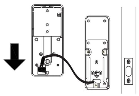
**Note:** Cable goes below deadbolt, The wire connectors can only be connected in one way. **Install back panel**
