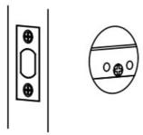
B If the bolt holes are centered in the door hole, no adjustment is required. Proceed to step 2. If the bolt holes are NOT centered, adjust latch. See "bolt Adjustment."
