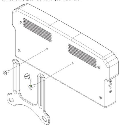
Replace the existing upper bolts which hold the motor in place with the countersunk ones included (A8). Use these bolts, including existing washers and locknuts to fix the mounting bracket to the front mount.
