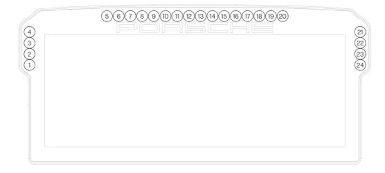
There should be enough info in the provided LED profile to be able to adjust to your liking. Just keep in mind, you mostly need two values. The number of the LED where you want an effect to start, and the amount of LEDs to use for said effect (in a clockwise direction).
