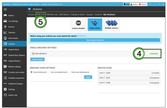
After we have confirmed the connection, press 'RGB Leds' (5) in the top row of options.
