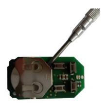
For battery change, the device needs to be opened by removing the three little screws on the backside of the device. Use a screwdriver or any other usable gently push out the battery as shown in the picture. During reassembly watch the position of the white rubber and make sure the silver buttons fit exactly in the nipples of the rubber.
