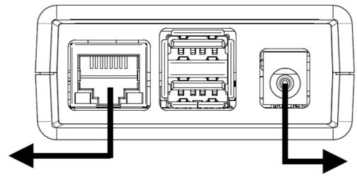
Use supplied RJ-45 cable to connect directly to router
