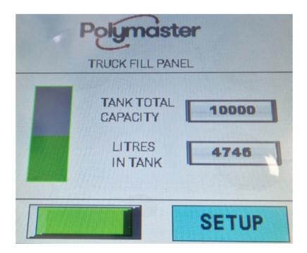
The SETUP screen is password protected so only authorised users can edit the controller's functionality. See the password section in Appendix 2 for these details. Click in the white box to enter the password.
