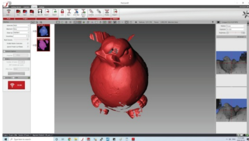
Figure 8: Sample of unsuccessful scan alignment due to lack of overlapping data or the orientation of the scan data to be aligned is wrong.
