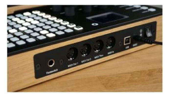
The Seq is equipped with a wide array of inputs and outputs. This allows communication with a wide variety of devices. The Seq also allows feeding tracks with MIDI notes using MIDI controllers. While looking at the back panel, from left to right, find:
