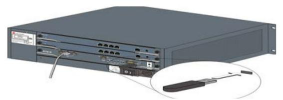
Power the RMX ON. The FAN STATUS and PWR STATUS LEDs turn ON. Wait for the upload process to complete. It is completed when all the flickering and
