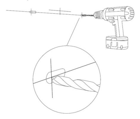
To ensure your holes are level with one another, drill your holes at the intersection of the vertical stud marks and the horizontal line you marked with the level.
