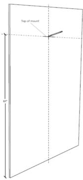
4. Locate studs in your wall using a stud finder and mark stud location by using a pencil. Mark your 2 studs a little below the line you drew in the previous step.
