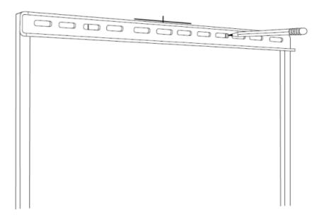
7. Using a level, draw a line between the two stud marks. Make sure your line intersects the center of both stud marks and is close to middle of the traced hole marks.
