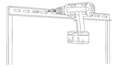
10. Now that the mount is in place, locate holes on the bottom of the mount that are in-line with holes you just drilled into and repeat steps 8 & 9.
