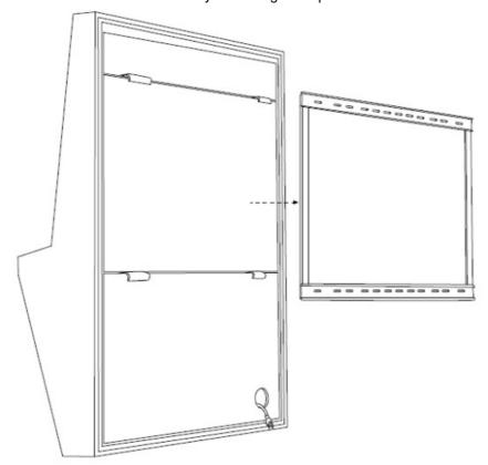
6. Make sure the mount is oriented with the correct side against the wall and hold it up to the wall. Line the top of the mount up with the first mark you made (in step 3). Hold the mount so that it is centered on the center line you drew, then move the mount left or right until you can see the pencil marks you drew to mark the center of the studs. Trace the inside of 2 holes where your stud mark lines are visible.
