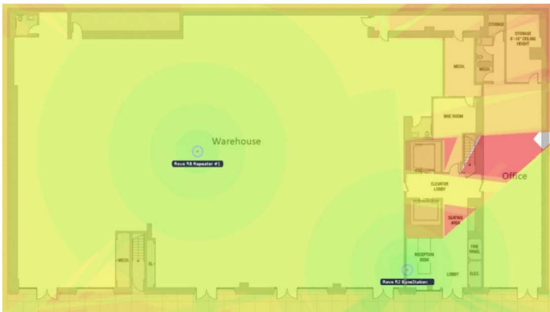
Floor plan example with one Rove B2 base station and two paired R8 repeaters
