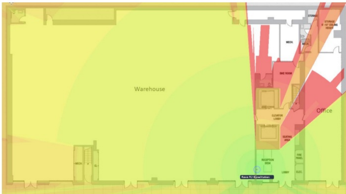
Floor plan example with one Rove B2 base station and one paired Rove R8 repeater
