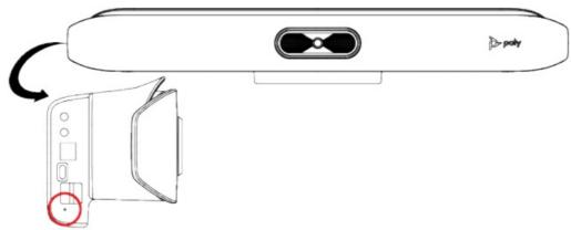
• On the bottom of the Poly Studio X30, insert a straightened paper clip through the factory restore pinhole.
