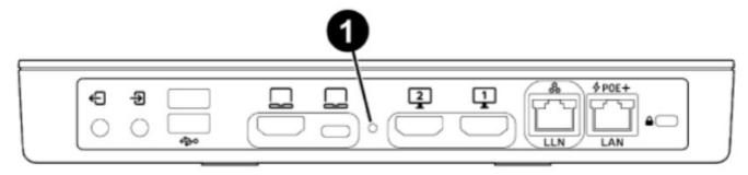
• On the front of the Poly G7500, insert a straightened paper clip through the factory restore pinhole.
