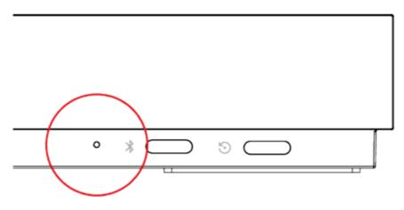
• On the bottom of the Poly Studio X72 or Poly Studio X70, insert a straightened paper clip through the factory restore pinhole.
