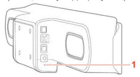
• On the side of the Poly Studio X50, insert a straightened paper clip through the factory restore pinhole.
