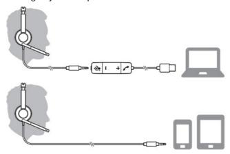
**IMPORTANT** Ensure that your 3.5 mm connector is fully connected to the headset controller.
