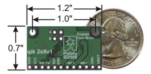
The qik 2s9v1 measures  $0.7" \times 1.2" \times 0.28"$  (17.8 x 30.5 x 7.1 mm) and weighs 0.07 oz (2.0 g) without the header pins installed. It has two mounting holes, one in each top corner. The holes have a diameter of 0.086" and are designed for #2 or M2 screws.
