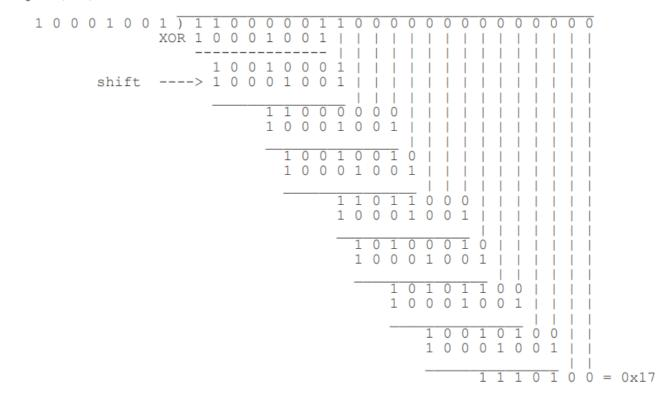
So the full command packet we would send to retrieve the PWM configuration parameter with CRC enabled is: 0x83, 0x01, 0x17
