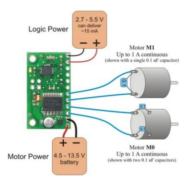
The Qik motor controller takes two power inputs: motor power supplied via the VMOT and GND pins at the bottom of the board and logic power supplied via the VCC and GND pins at the top of the board.
