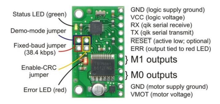
The Qik connections are shown above, and most of the pins are labeled on the back side of the motor controller. All square pads are ground.
