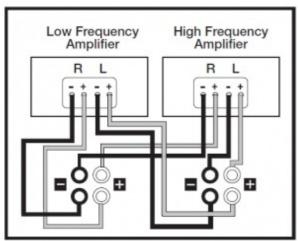
Bi-amping, or using separate amplifiers for the low and high frequency sections of your speakers. Remove flat metal jumpers.
