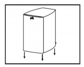
Slide the speaker down on the screw head to catch the keyhole slots.
