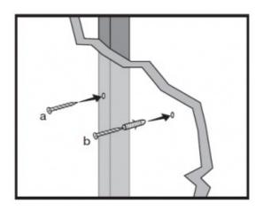
Use #10 panhead screw for wall stud (a), use #10 wall anchors with appropriate weight rating + screw for no wall stud (b).
