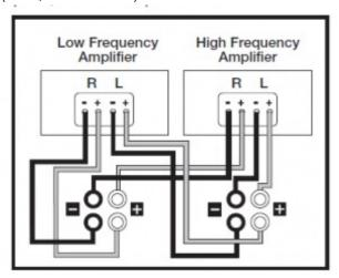
Bi-wiring, or using separate speaker wire connections for high and low frequency sections. Remove flat metal jumpers.
