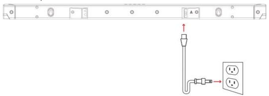
Position the subwoofer and connect it to an AC outlet. For best performance, place it on the same wall as the TV.
