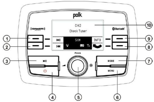
Press the MODE button (7) to enter mode selection display. Press the SXM soft button (9) to change to SiriusXM mode.
