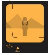
For an in-focus, off-center subject: keep the button half-pressed, re-aim the autofocus frame, and shoot
