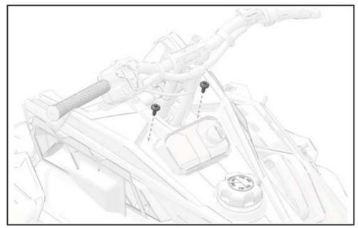
6. Install two screws and one push pin rivet. Torque screws to specification.
