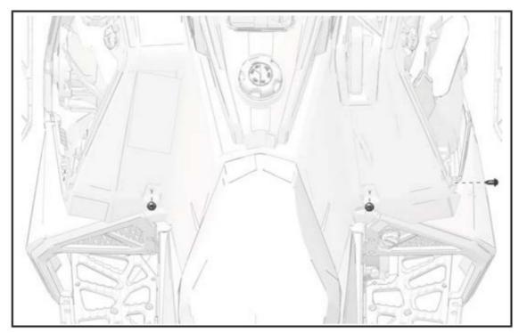
4. Remove and keep secondary clutch tool.
