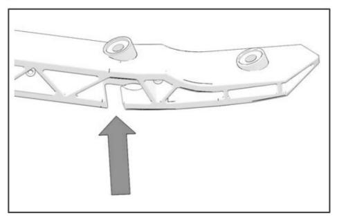
5. Attach handguard accent light using two kept screws. Tighten until fully-seated.
