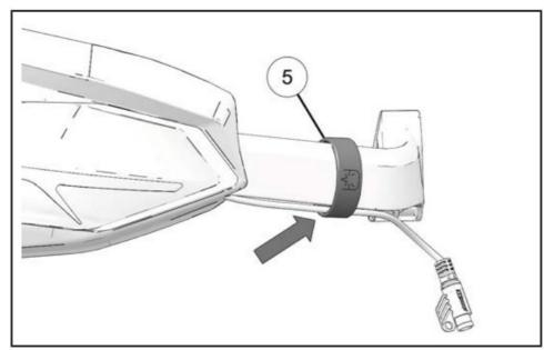
7. Install handguards onto handlebars. Put handguards next to handlebar riser. Torque screws to specification.
