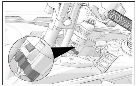
7. Remove two clips and disconnect switch panel from cowl. Move switch panel away from cowl. Lift cowl away from snowmobile and set to right side. Leave starter pull handle attached.
