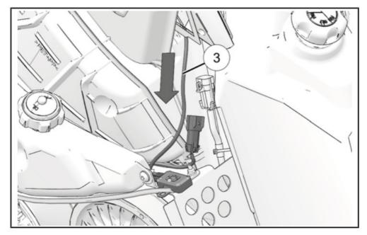
11. Remove existing nut from top of clutch guard.
