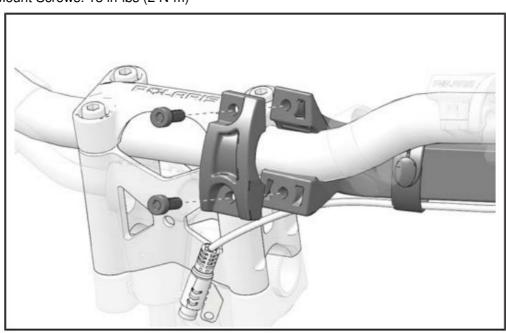
8. Route handguard accent light wiring along steering post. Connect to harness 3.
