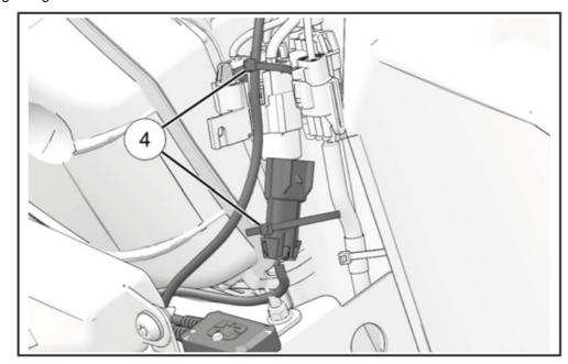
14. Attach harness to chassis tube using cable tie 4.
