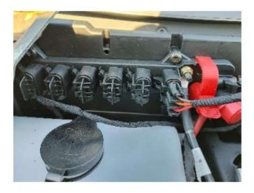
5. Find the 2 pin plug under the bed, near the throttle body, remove the cap and connect the 2 pin connector included with the kit, route the wire through the hole at the bottom of the drivers side rear roll cage and rear firewall, secure the harness along the vehicles main harness with the supplied zip ties.
