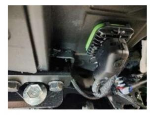
7. This kit does not include lights unless chosen at the time of purchase. Pod lights can be mounted to the outer roof bolts, remove the roof bolts, install the pod light bracket loosly on the pod light, route the connector between the roof and rear roll cage, make sure the wires are as far away from the bolt as possible to prevent pinching, install the roof mounting bolt through the mounting bracket and reinstall on the machine, adjust the pod light angle and tighten the bracket bolts.
