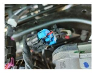
6. Route the brown wire to the top of the roll cage where the other wires are, install the Y harness along the top of the rear roll cage, connect the bullet connectors to their matching colors.
