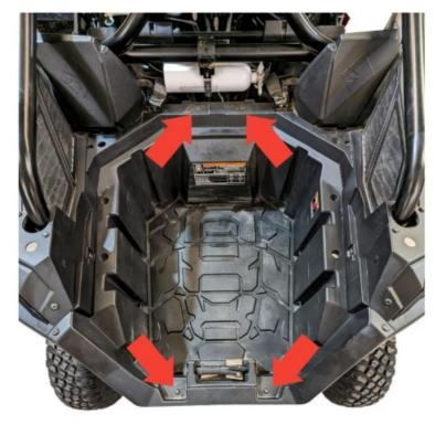
• Install two of the factory torx bolts loosely into the holes nearest to the seats and then install the 6mm bolts and washers into the two mounting holes towards the rear of the vehicle. Do not tighten down any of the hardware at this point.
