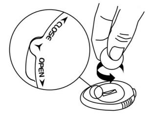
2. Place the battery (CR2430) inside the cover with the positive (+) side facing the cover (picture 3). Make sure the sealing ring is in the groove.
