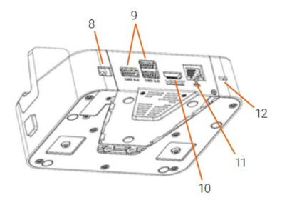
8 Power supply connector 9 USB 3.0 ports\* 10 HDMI port\* 11 LAN (RJ45) port\* 12. Kensington Lock hole
