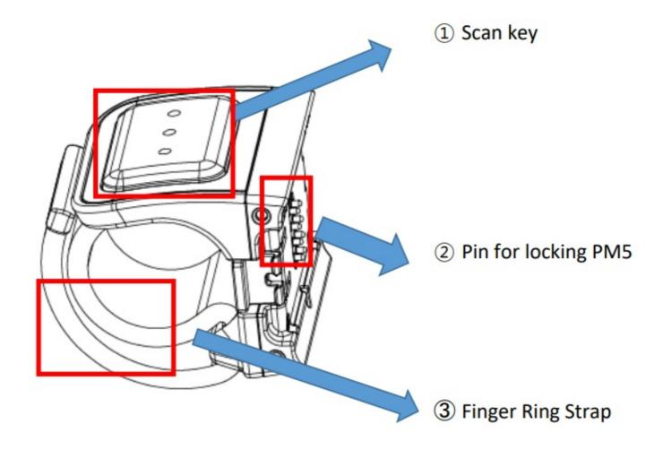
PM5 can connect with single trigger. Single trigger has a finger strap so user can put PM5 on their finger.
