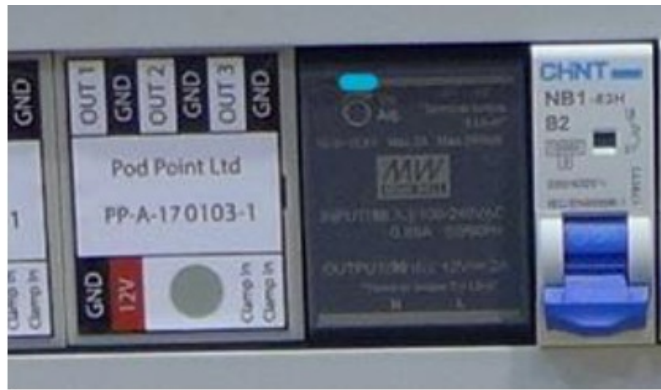
Array controller PSU indicator lamp (normal).
