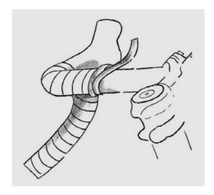
Remove bar tape to expose the bare handlebar and cable housing/wiring for proper clamp placement
