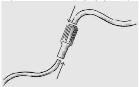
Insert cable originating at the dropper post through the rotary ferrule and through the housing to the lever
