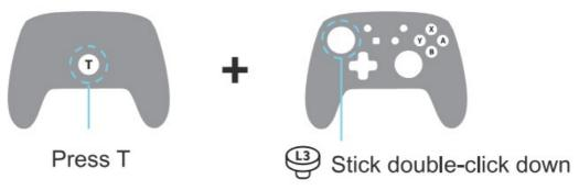
3. T plus L3 (stick long press for 2 seconds) adjustable light brightness, light scheduling a total of levels, 25%,
