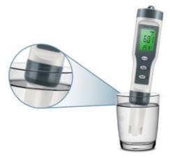
**Note**: The liquid should not exceed the water level line.
