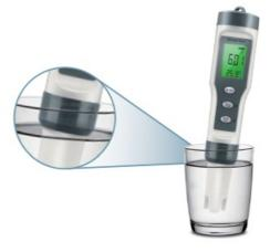
**Note**: The liquid should not exceed the water level line.
