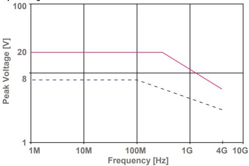
——Dynamic Measuring Range ---- Maximum Input Voltage
