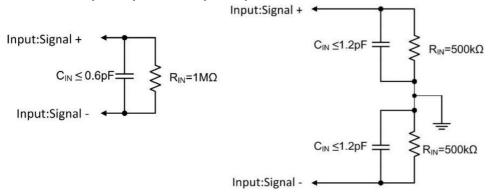
The HSDP-Series uses a PMK custom high speed FET input amplifier that provides a superior high frequency response, as well as low noise and low distortion to accurately capture the signals being measured.
