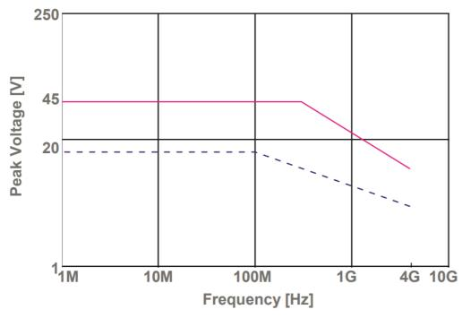
——Dynamic Measuring Range ---- Maximum Input Voltage
