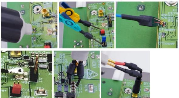
The input offset capability extends the input range of the probe. Having an input capacitance of <0.6pF || 1M $\Omega$  between the probe tips, allows the HSDP Series to be used to probe sensitive circuits without adversely loading the circuit under test.
