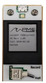
The LCD Screen shows the status of the miniDOT Clear Logger. The screen will display information as long as the AA batteries are installed. When the Logger Control Switch is in HALT, the screen displays the miniDOT serial number, operating system revision, calibration date, and status ("Halted")
