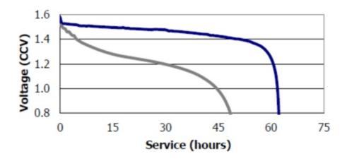
The figure to the left gives a general idea of terminal voltage vs. lifetime. Service life in hours is incorrect since miniDOT Clear Logger draws far less than 50 mA continuously, but the general shape of the voltage vs. time gives an estimate of life remaining. This plot is taken from the manufacturer's specification. The plot is for a single battery. The miniDOT Clear Logger halts operation at a total of 2.4 Volts.
