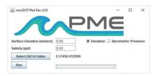
The miniDOT Plot program plots the files recorded by the miniDOT Clear Logger. The program reads all the miniDOT Clear Logger files in a folder, except the CAT.txt file. The program will also compute air saturation from the dissolved oxygen measurements. To do this, the program must know the air pressure and salinity. It calculates air pressure based on elevation of the water surface above sea level or uses the barometric pressure you enter if Barometric Pressure is
