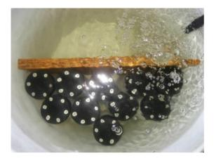
Record measurements for several hours or a day, but in any event long enough for the miniDOT Clear Logger's temperature to come to equilibrium with the water. During the experiment, find the local air pressure, either from measurements or from a local weather station. Watch out... weather stations often report barometric pressure referenced to sea level. You must determine the absolute barometric pressure at your elevation.
