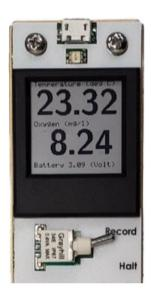
The USB Connection allows communication between the miniDOT Clear Logger and an external HOST computer. When connected, the miniDOT Clear Logger is in HALT mode regardless of the Logger Control Switch position. When disconnected, the miniDOT Clear Logger's mode is controlled by the Logger Control Switch position. The switch position may be changed while the USB is connected.
