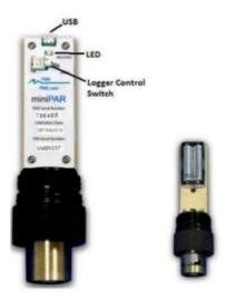
Removal of the cover reveals the miniPAR Logger's connections and controls, shown here. The LED Light is a LED that can display either red or green light. This is used to indicate the different features described in Chapter 1 of this manual. The Logger Control Switch controls the miniPAR Logger's mode:
