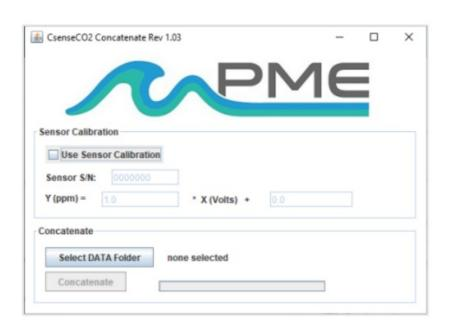
Begin the program operation by clicking "CsenseCO2Concatenate.jar". The program presents the screen shown below. CsenseCO2Concatenate reads and concatenates the files recorded by the C-sense Logger. The software produces CAT.txt in the same folder as selected for the data. CAT.txt contains all the original measurements and contains two additional statements of time. If the Use Sensor Calibration is checked the CAT file will contain an
