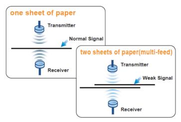
The ultrasonic sensor detects the Multi-feed of original documents during scanning. The ultrasonic function can be turned on when scanning document with labels, sticky notes, or taped receipts. This innovative design prevents Multi-feed and e ectively scans documents of di erent weights or thickness. Thanks to Multi-feed prevention, optimum reliability is assured even when scanning high volumes of documents.
