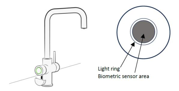
Power the tank, a beep will sound and the ring on the tap flashes green. Present the registering tool from below as shown in the drawing and keep pressed until you hear two short beeps (keep pressed 5 seconds more). The ring flashes red/green and the tap emits a series of beeps indicating that it is in programming mode, remove the tool.
