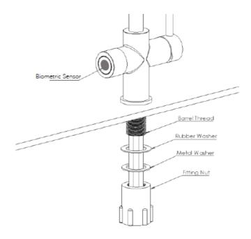
Feed the tails through the barrel thread and hand tighten into the tap. Fit the tap in the desired location using the black plastic fitting nut.
