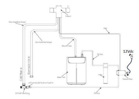
Install the Solenoid valve close to the boiler with 4 screws and connect it as shown on the drawing. Insert the connector from the sensor cable into the solenoid valve box and connect the 12Vdc input to the 12V power supply Socket on the rear of the boiler tank.
