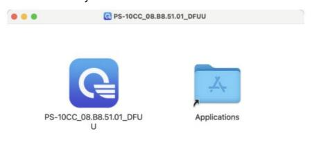
6. When the firmware update utility launches it will check for connected charging stations and show the status of the component firmware to be updated.
