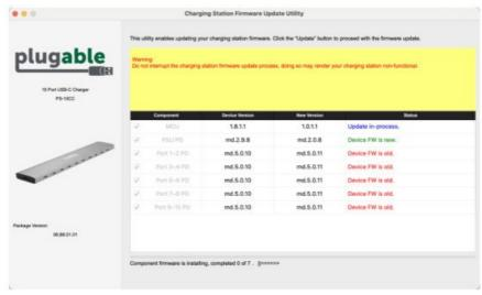
8. The updater will progress through the various components in the charging station in turn updating each component with a progress bar at the bottom of the updater,
