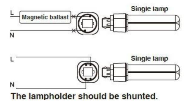
When used with a magnetic ballast, cut all wires connected to the ballast. And the PLC can not plug in a 2 pin G24D or GX24D lampholder. Modify the lamp holder to a G24Q or GX240, meanwhile shunt the lamp holder.
