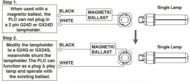
The lampholder should be shunted.
