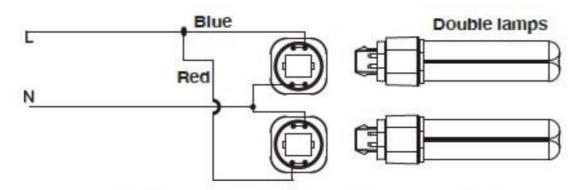
The lampholder should be shunted.
