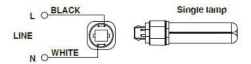
The lampholder should be shunted.
