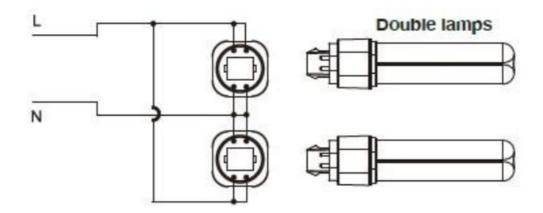
**Diagram 4 – Electronic Ballast Fixture Wiring Modification**
