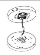
• 5. Feed all wire up into the battery backup box and raise the lighting fixture up to the ceiling. Align the edge of the fixture with the ball bearings on the mounting bracket and press until it pops and locks into place.
