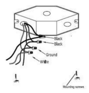
2. Screw the emergency backup unit up into the junction box using the  $2\times8/32$  screws provided. Then using the wire unit provided, connect the t hree cables available for connection into the junction box.
