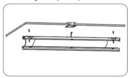
5. Wire to the main supply power though the junction box.
