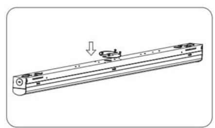
3. Separate the module board from the fixture base.
