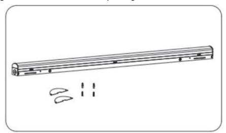
2. Attach the junction box covers to the fixture.
