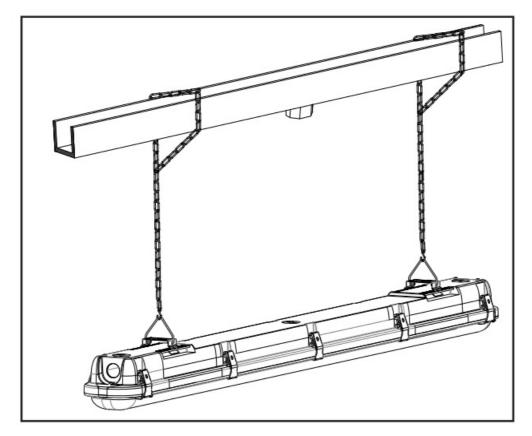
4. Release latches by pulling top of the latch away from the housing. Set the lens aside.
