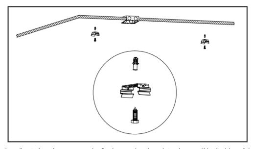
2. Secure mounting clips to housing recesses by firmly pressing them into place until both sides of the clip are
