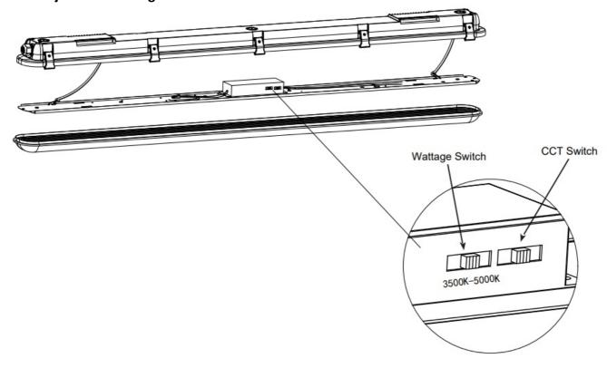
The end users may adjust the color temperature and lumen output respectively by the two DIP switch buttons integrated into the driver. Each DIP switch is accommodated with 3 options (left, middle and right), corresponding to 3 color temperatures and 3 wattages respectively, which can perform the desired color temperature and lumen output combination.
