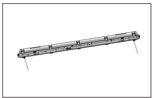
9. Secure lens to the housing with lens latches.
