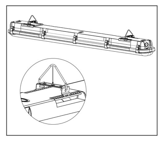
3. Hang fixture from the customer-supplied chain using V-brackets.
