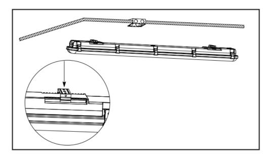
3. Release latches by pulling top of the latch away from the housing. Set the lens aside.
