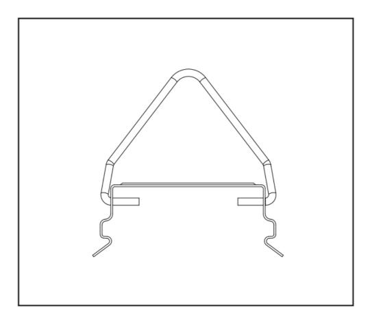
2. Secure mounting clips to housing recesses by firmly pressing them into place until both sides of the clip are secured.
