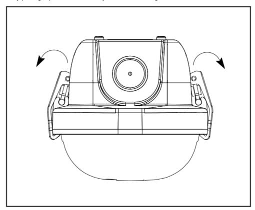
5. Without touching LED boards, detach LED tray from the fixture. Safety cables will suspend the tray.
