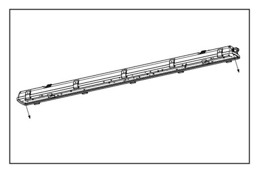
6. Assemble the PG13.5 waterproof cable connector and position it in the appropriate end of the fixture housing. Bring an (owner-supplied) 6-10 millimeter diameter electrical cable through the PG13.5 waterproof cable connection. Include 0-10V dimming conductors in the cable if 0-10V dimming is desired. Make appropriate electrical connections with the driver.
