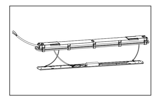
Include 0-10V dimming conductors in the cable if 0-10V dimming is desired. Make appropriate electrical connections with the driver.
