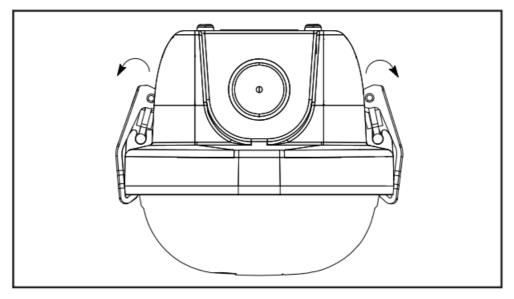
4. Without touching the LED boards, detach the LED tray from the fixture. Safety cables will suspend the tray.
