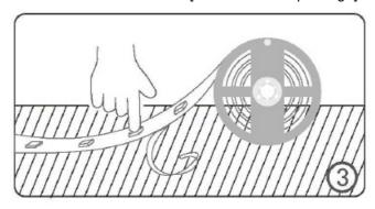
4. Tear off the back tape and paste the strip to the surface smoothly and correctly. Connect the LED strip to controller and driver based on the diagram.
