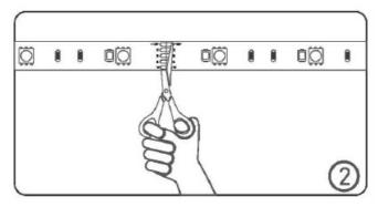
3. Measure the length required on the surface and cut the LED strip accordingly. Once the LED strip is cut, both ends will need separate power sources and connectors[Not included in package].
