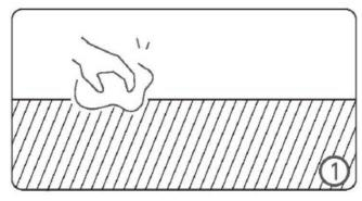
2. Using alcohol prep pad to clean the surface on the installation place, make sure it's clean, dry and smooth, Or it will reduce the adhesiveness of the back tape. Remember the back tape could be only used one time. The LED strip will fall off if the surface is not in good condition or the back tape is reused.
