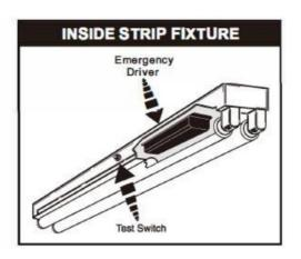
Refer to the illustrations above and install the test switch through the driver channel cover of a troffer or through the side of a strip fixture.
