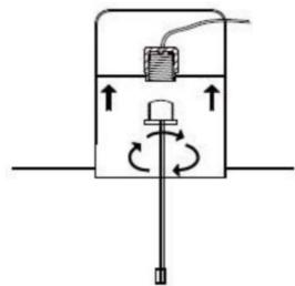
**Step 6**. Select your desired CCT by sliding the switch on the top of the disk light to the desired setting. Then connect the fast connector between the recessed housing and the disk light.
