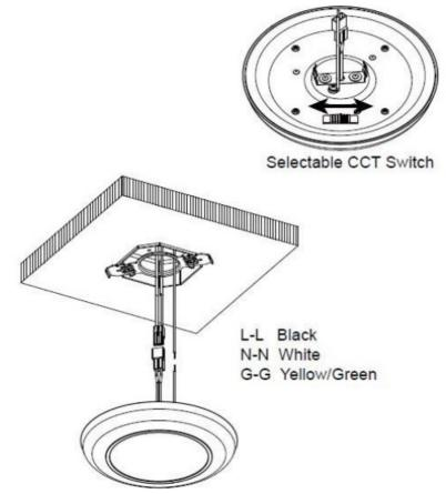
**Step 6.** Check if the wires are well connected and put them inside of the junction box, then attach the disk light to the multi-functional bracket.
