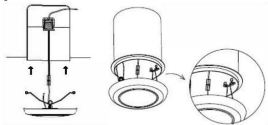
**Step 8**. Push the disk light into the recessed housing, making sure it's firmly attached. Then turn on the power to verify your successful installation.
