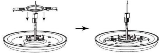
**Step 3.** Take out the spring tabs and screws and install them on the disk light.
