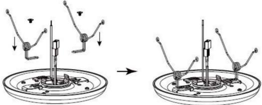
**Step 4**. Loosen the screws on the bracket to adjust the spring tabs so they can fit 5 or 6-inch cans. If the can is 4-inches, the spring tabs need to be rotated 180°. Once the spring tabs are in the right position, tighten the screws on the bracket.
