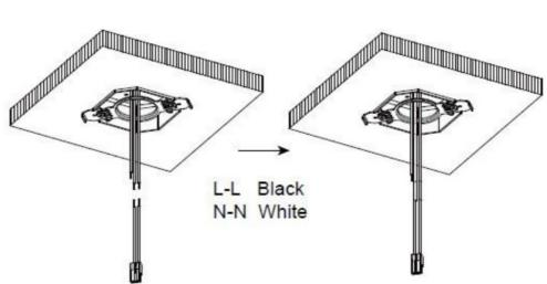
**Step 5.** Select the desired CCT by sliding the switch on the top of the disk light to your desired setting, then connect the male and female fast connector between the disk light and junction box. Use a wire nut to connect the ground wires.
