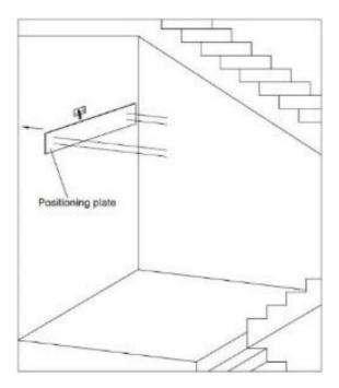
5. Screw four mounting screws into each anchor bolt, then connect the AC wires.
