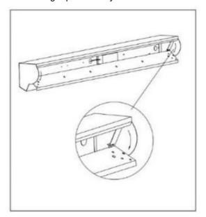
4. Install anchor bolt. Drill four holes in the corresponding position on the wall using the positioning plate provided by the manufacturer. Insert an anchor bolt into each hole.
