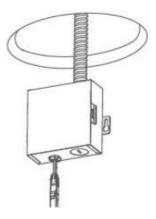
7. Push the spring clips and insert the fixture into the hole in the ceiling.
