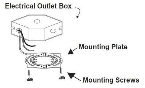
2. Connect the supply wires on the fixture using wire nuts or push the wires into a Quick Connector. Connect white to white, black to black, and copper wire to copper wire as the ground connection.
