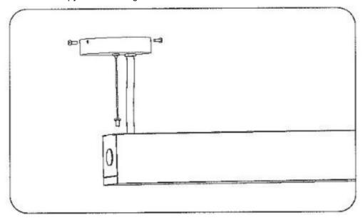
5. Hang luminaire. Screw both bottom parts of the cables clockwise and secure them on the top of the housing. Make sure the light is securely hung.
