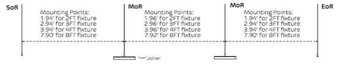
Screw the joiner "-" to the MoR aircraft cable in turn.
