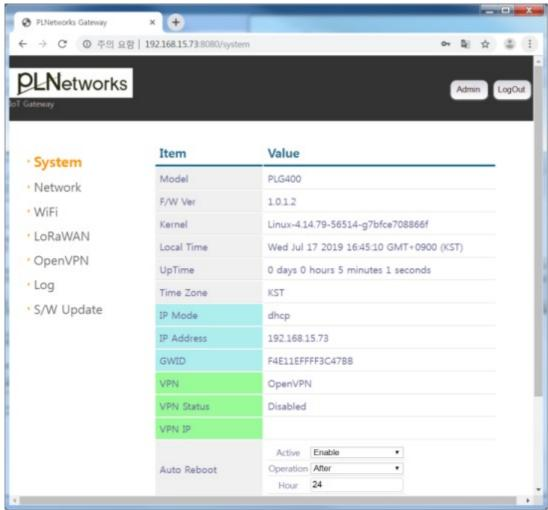
Shows the model and network, firmware and kernel versions currently reflected in the PLG400.
