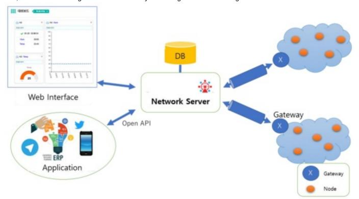
LoRa Gateway is located between the Node and the Network Server system and converts the sensing data provided by the Node into a Network Server compatible format and transmits the commands sent from the Network Server to the Node. Usually, a Linux router with wired (Ethernet) and wireless (Bluetooth, LoRa, ZigBee, etc.) communication interfaces based on processors such as ARM Cortex-A series and MIPS.
