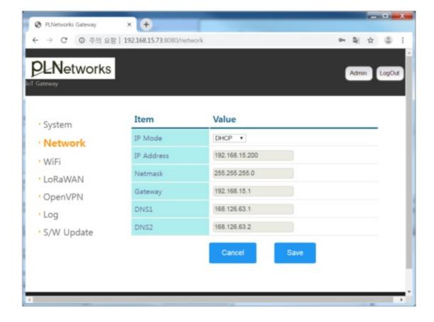
The displayed parameters represent the values currently set in the PLG400. Set the IP address that the PLG400 will use to connect to the WAN.
