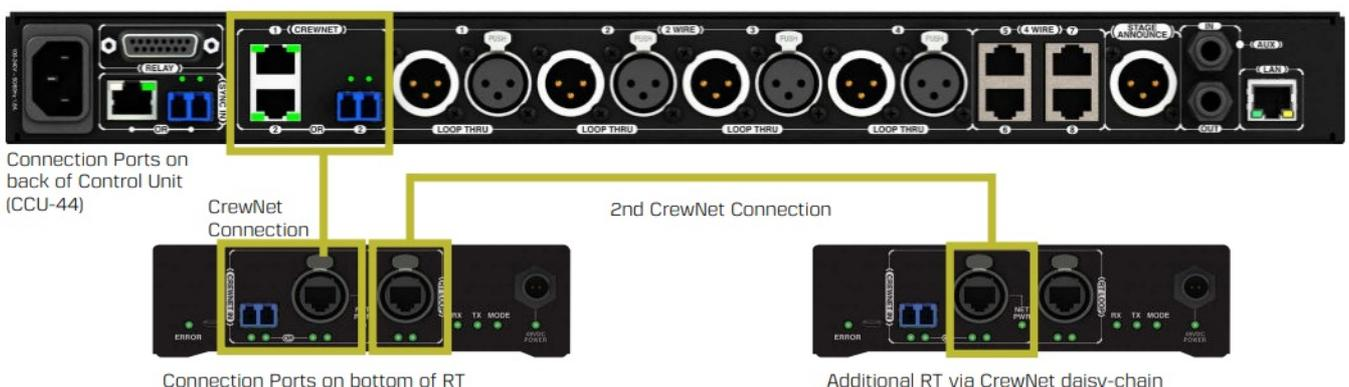
Connection Ports on back of Control Unit (CCU-44)
