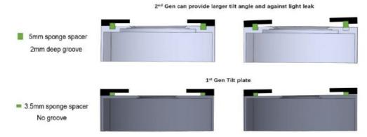
When taking solar photographs with a prominence telescope, the Newton ring is annoying. A smoother solar image without a Newton ring could be taken by adjusting the focal plate. Get a much smaller field curvature of the telescope.
